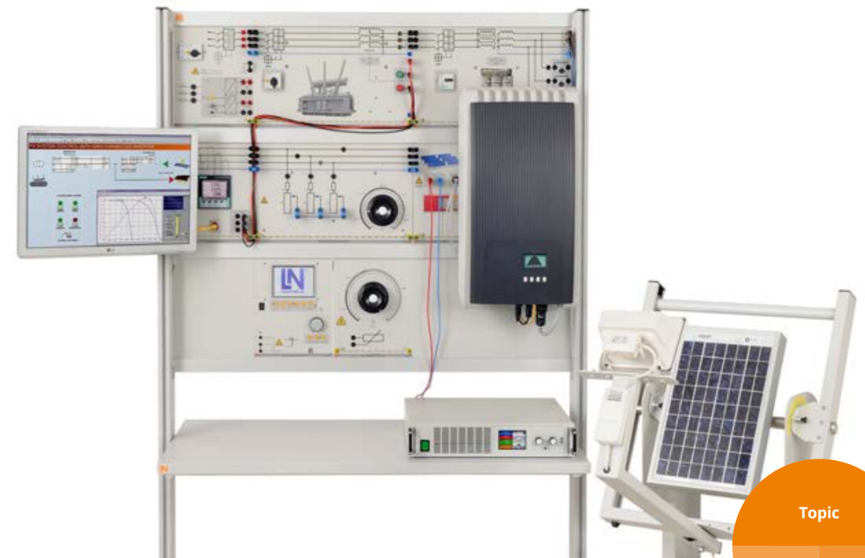
Sample experiment from "Set-up of photovoltaic systems in operation parallel with mains grid" EPH 3
